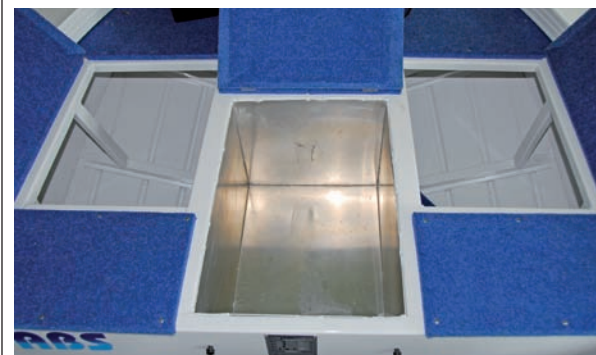
Large side storage compartments adjoin the large live well up front of the Bullshark. All are accessed via finger tab hatches.
