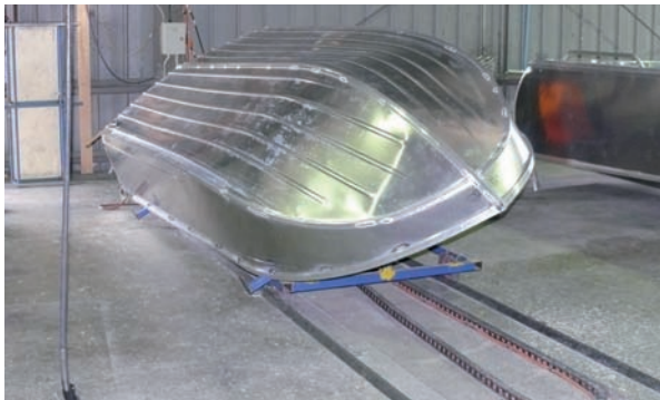
A barra's view of the Bullshark's hull: note the strong pressings.
