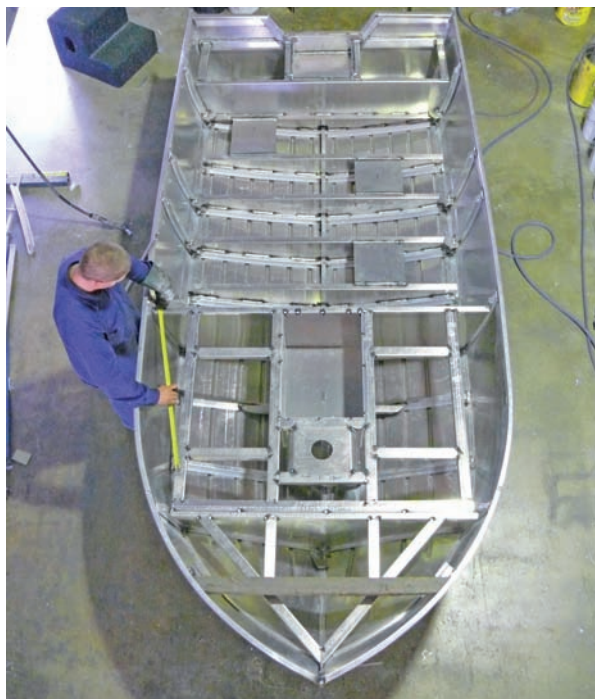
Rigidity within the extra strong framework is one feature that should ensure a long working life for the Bullshark P420.
