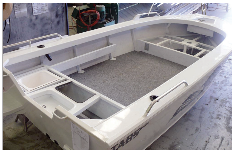
This factory image shows the layout of the TABS Razorback 440 before flooring has been added. (Dean Wilson image)
